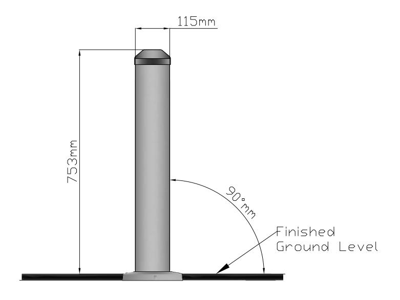
B4.D Fixed Galvanised Bollard Bollards.co.nz sales@bollards.co.nz
