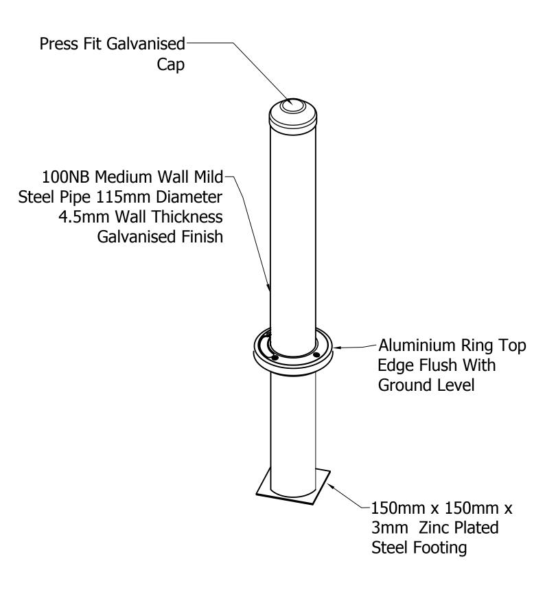
B4.D Fixed Galvanised Bollard Bollards.co.nz sales@bollards.co.nz
