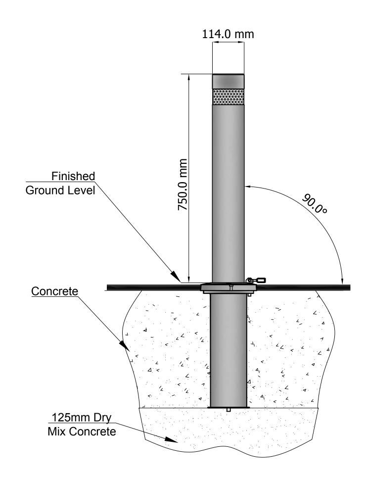
B2.F Self-Righting Removable Bollard Bollards.co.nz sales@bollards.co.nz
