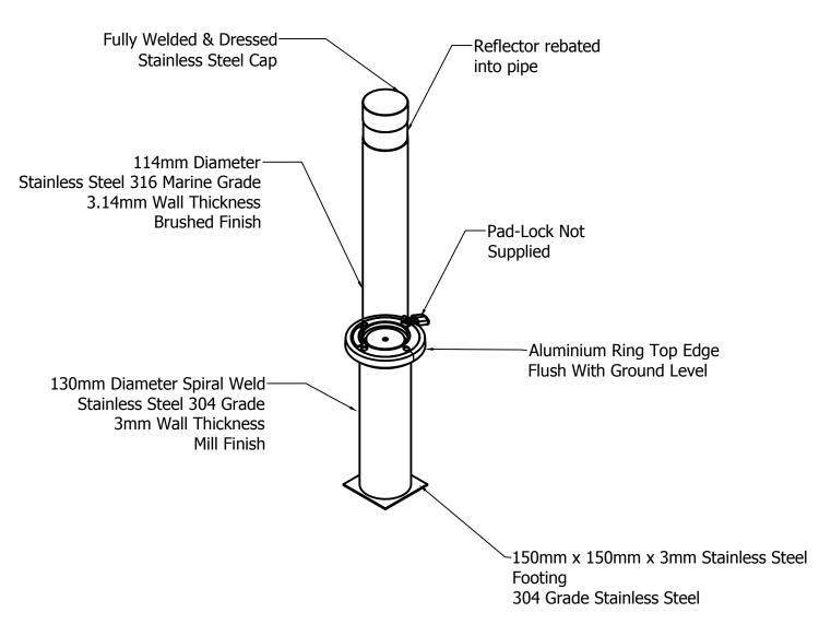
B2.F Self-Righting Removable Bollard Bollards.co.nz sales@bollards.co.nz
