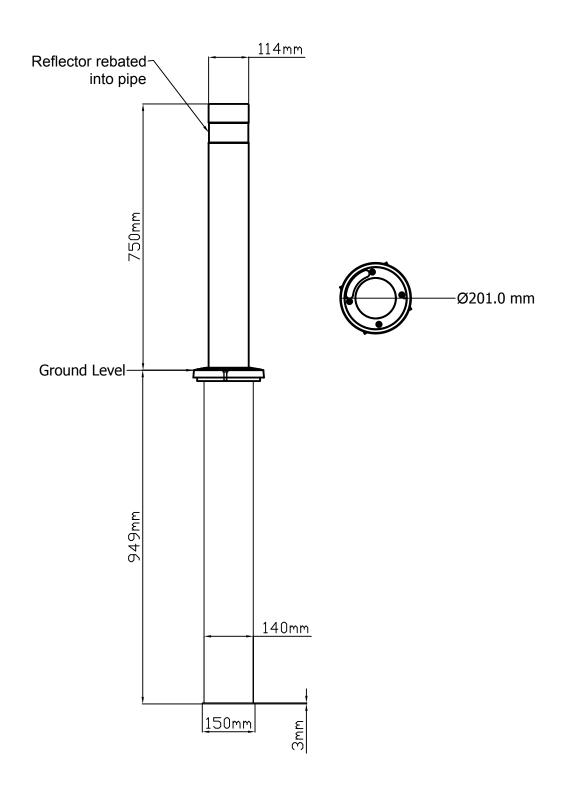
B2.B Self-Righting Retractable Bollard Bollards.co.nz sales@bollards.co.nz
